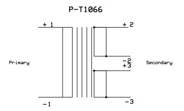
The transformer is DC gapped and has 3 identical 150ohm windings that are trifilar wound. So can use as 1:1:1 or 1:2 or 2:1 applications.
