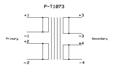
The transformer is DC gapped and has 4 identical 150ohm windings that are trifilar wound. So can use as 1:1:1:1 or 1:2, 2:1, 3:1 applications.
